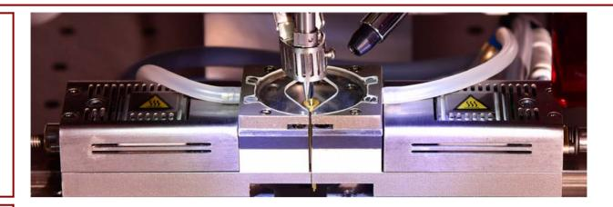
The **TO** - **HEATING UNIT** is a high-speed heating system, tailored for eutectic applications on all types of TO housings, up to a diameter of 30mm. It can be added to any **TRESKY** system of the **T-300X** Series. The sophisticated design of the TO- heating unit allows quick change over from one TO size to an another or to smaller substrates/arrays. The bonding area can be surrounded with inert gas and is switched automatically on/off during the process.
