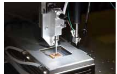
2nd spindle for preform pick-up
