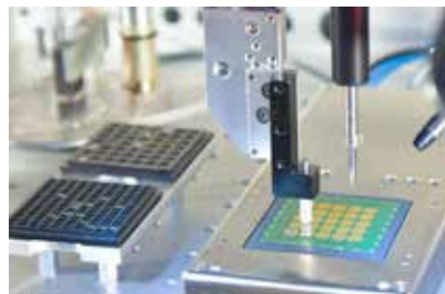
Stamping unit for adhesive application
