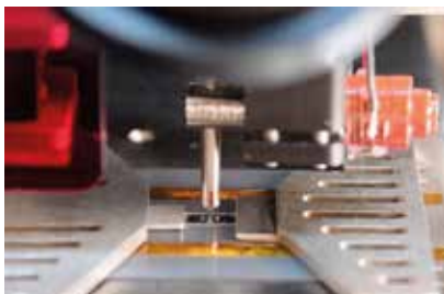
Scrubbing motion or Ultrasonic bonding action
